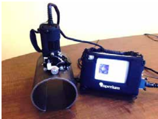
Figure 1. Acoustocam™ with encoder and dual-element transducer on an 8" pipe.
