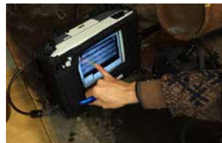
Figure 12. Inspector identifies thin area of 6" steel pipe using the 2-D C-scan as a guide.
