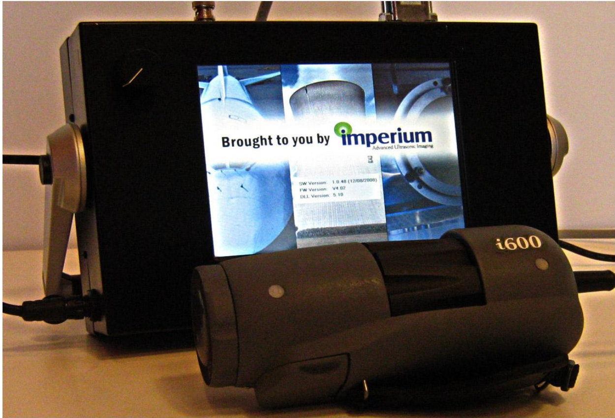
Figure 1. Acoustocam Ultrasound Imaging Camera and controller unit. (Image courtesy of Imperium Inc.)
