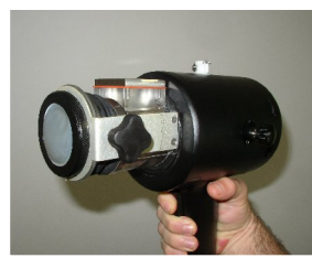
Figure 4: New Handheld Ultrasound Camera for rapid inspection of materials with LCD
