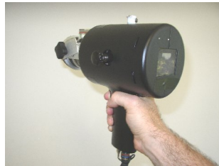
Figure 4: New Handheld Ultrasound Camera for rapid inspection of materials with LCD
